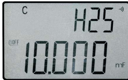
Compare mode in the U1701B reduces test set-up time for capacitor sorting.
